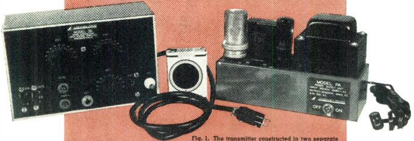
Fig. 1. The transmitter constructed in two separate units: transmitter proper and power supply.
